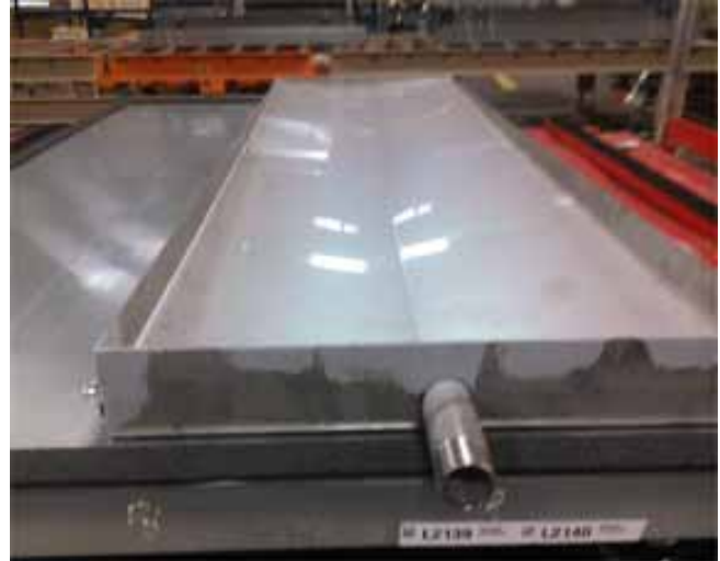
Figure 12. Base panel with wall and roof panels removed.
